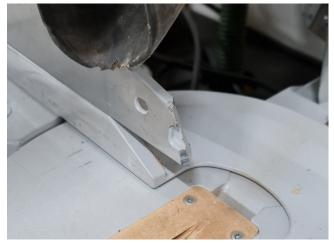
Unfortunately damage has occurred to one of our machines - the Festool Kapex compound mitre saw. The left rear alloy stop has been cut through when someone carelessly cut at an angle. Thankfully, it does not seem that the blade has been damaged, however, the replacement cost of this rear stop is \$156 from Festool.
